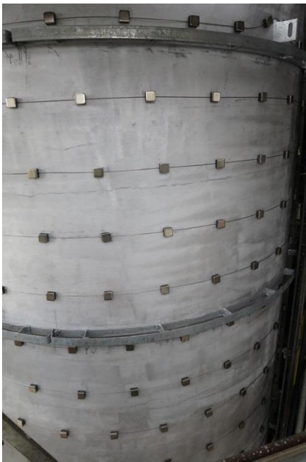
The fibre optic sensor cable (protected by a stainless steel tube) is fixed on the surface of the vessel with high temperature resistant magnets.
