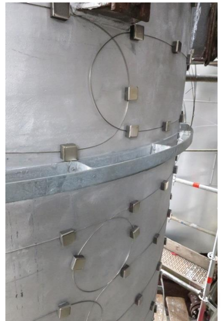
The fibre optic sensor cable (protected by a stainless steel tube) is fixed on the surface of the vessel with high temperature resistant magnets.
